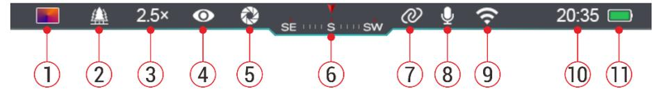
The status bar is located at the top of the image interface and displays the information related to the current operating status of the device.
